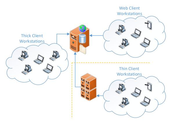
This diagram shows a fully scaled Suite network footprint. This installation uses (1) a file server for storing document repositories and our installation applications used to administer your installation. A separate server is used for hosting the database. Optionally one or more web servers for hosting Desktop Web Access. Optional use of one or more Terminal Servers or Citrix servers in a load balanced configuration.
